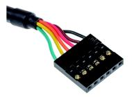
Figure 1.2: UART cable connector.
