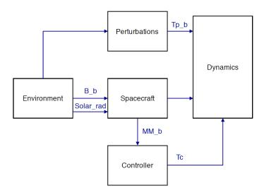
Figure 2.2: UPMSat-2 ACS high level model view.
