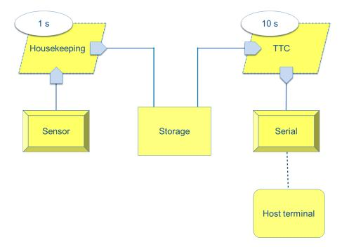
Figure 1.1: Software architecture of OBSW.
