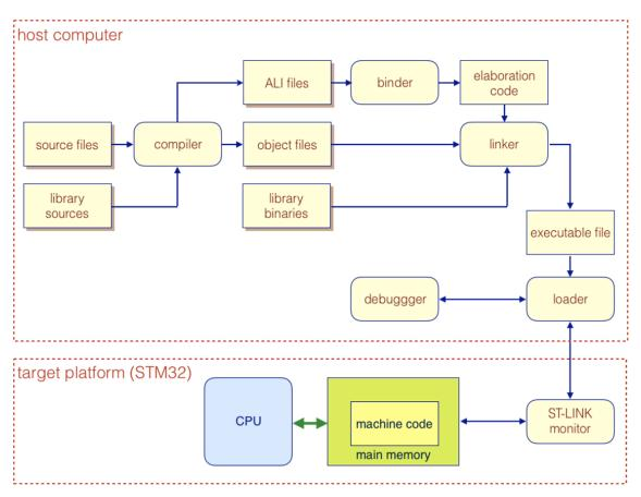
Figure 5: Cross-compilation and debugging system
